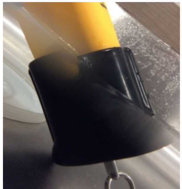
Figure 11: HPS1 production endcap installed on a Biomark R601 reader partially submerged in water.
